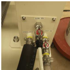
Pad cut rate measurement device (top) ... Neslab heater & chiller (center) ... Araca APD – 800 platen heating and cooling interface hardware (bottom)
