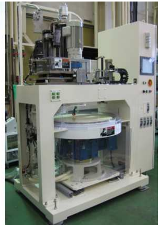
APD – 800 (300-mm polisher with automatic platen heating and cooling, 10-zone conditioner and in-situ frictional and pad temperature sensor)
