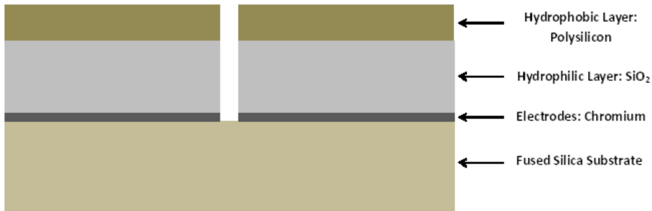
Multi-material electrochemical residue sensor
