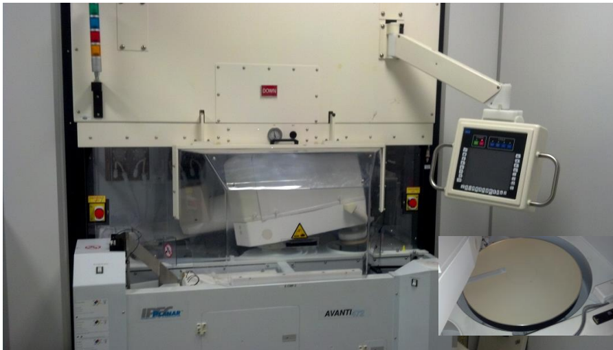
IPEC Avanti 472 CMP. Inset shows polishing pad/surface
