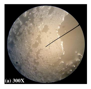
Assembly of 15 micron polyurethane beads on PC counterface at pH 7 (post UPW rinse) (a) monolayer rafts (b) & (c) continuous bilayers
