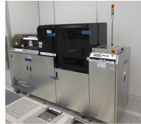
IPEC Avanti 472 CMP. Inset shows 8” polishing pad/surface (right) Lam DSS-200 Series II Brush Cleaner for post-CMP cleaning
