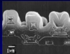
1000 nm Two Al Metal layers, BPSG
