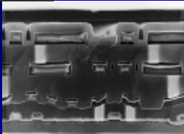
500 nm ILD planarization, W plugs w etch back
