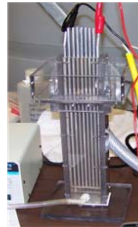
One-half m³/day bench-scale EC reactor with aluminum electrodes attached to a power source.
