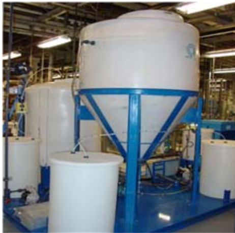
View of pilot skid with clarifier in the foreground, influent tank in left background and reactor in right background.
