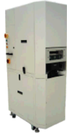
A full-wafer high pressure CO 2 processing tool (DFP 200, BOC Edwards) located in the laboratories of Watkins at UMass.
