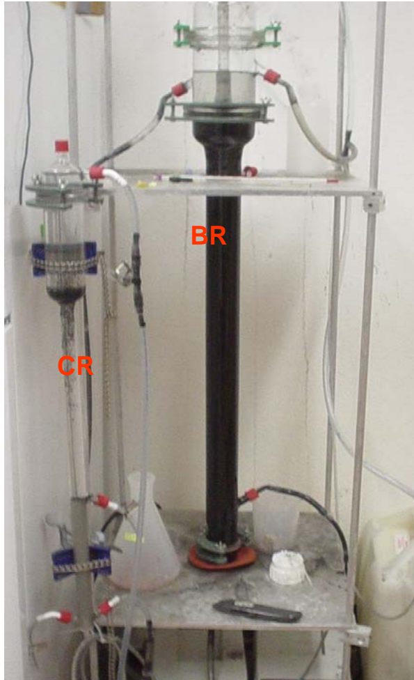
Photograph of the two reactor system used in this research. (BR) Anaerobic bioreactor; (CR) Crystallization reactor packed with sand
