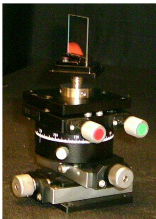
Figure 1. The 5-axis beam splitter positioner provides hardware alignment.
