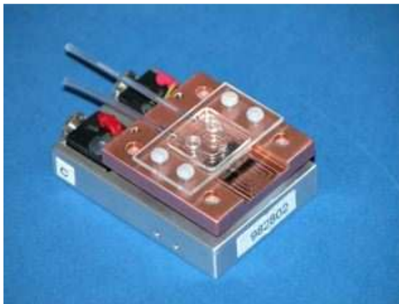
Figure 1. CMOS chip packaging for integration of fluidic substances with a CMOS chip.
