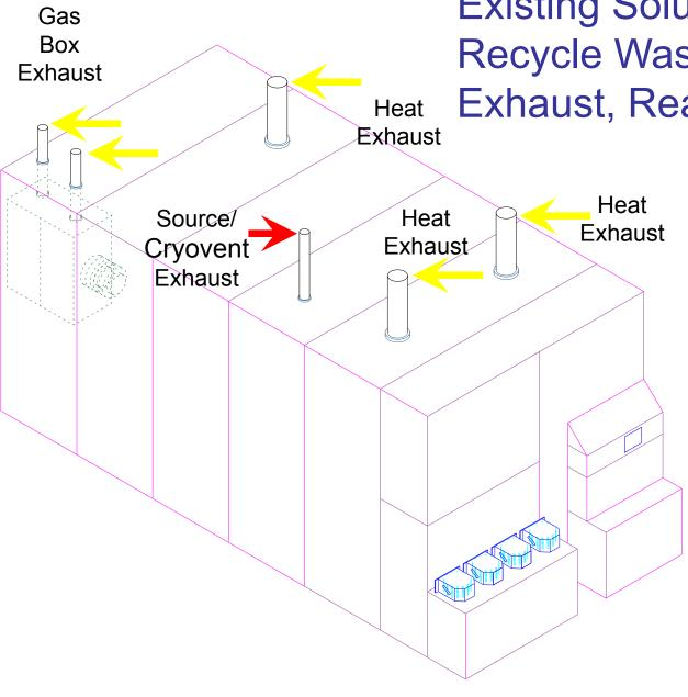
Existing Solution – Recycle Waste Heat Exhaust, Reactive
