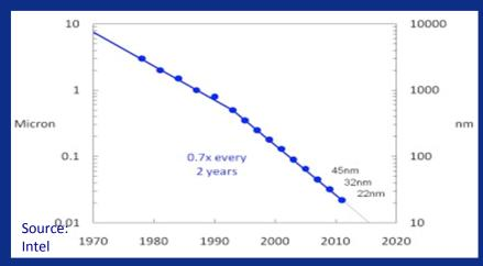
Moore's Law: Transistor dimensions scale to improve performance, reduce power and reduce cost per transistor
