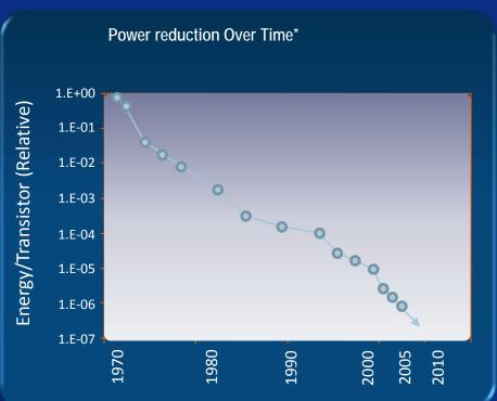
Each transistor in Intel's newest 45 nanometer processors uses 1/7000th of the power compared to our earliest transistors. If automobile fuel efficiency had improved at the same rate, today's cars would get ~100,000 miles per gallon.
