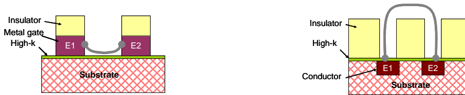
Figure 1: sample AC Impedance test structure for in-situ rinse and dry monitoring for the Gate First process (left) and the Gate Last process (right). The path followed by the current between the two electrodes of the test structure is shown as a solid gray line.
