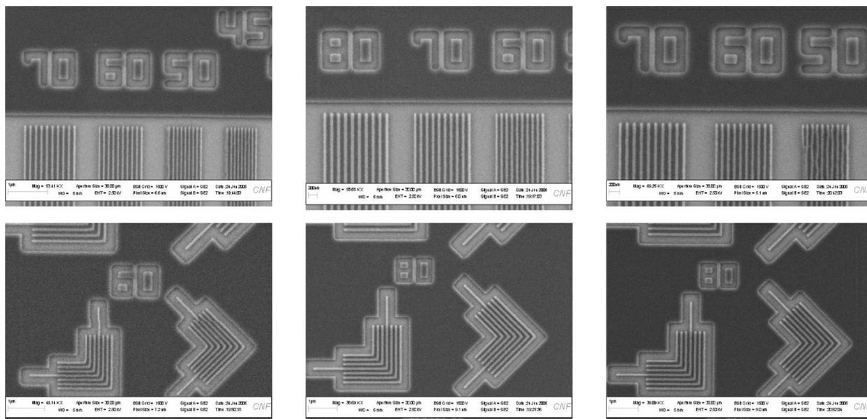
Figure 7. Top-down SEM images of resist films of poly(GBLMA-co-MAdMA) blended separately with TPSGB (left column), TPSNB (middle column), and TPSPFBS (right column) patterned by EUV lithography.
