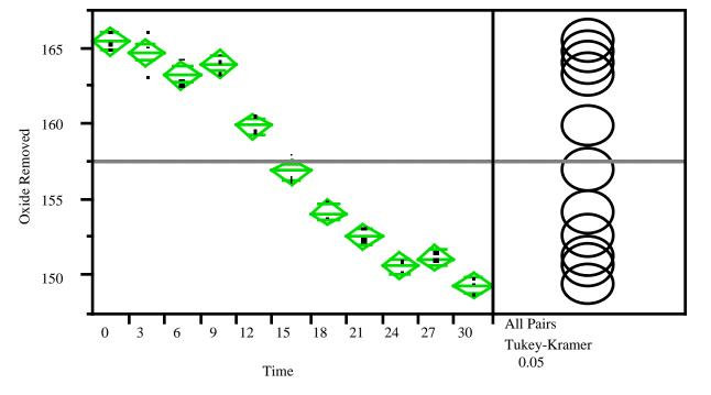
Processing wafers through a dilute HF bath causes change in etch rate over time
