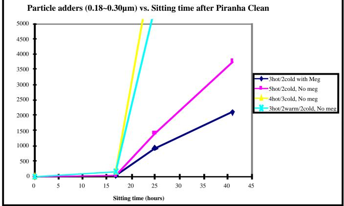
Particles will grow on the wafer surface after a Sulfuric-peroxide Clean
