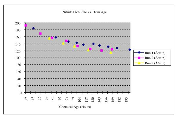
HF is used for removal of Nitride from dummy and test wafers in the fab. Assuming we etch the wafers for a long enough period, no problem should result from using the bath for 1 week
