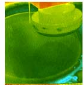
(b.) Carrier begins lowering the wafer onto the polishing pad for planarization.
