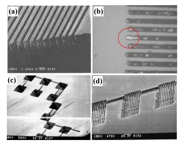
SEM images of µ-channels and µ-chambers carved on glass slides using femtosecond pulsed laser micromachining. (a) Grooves, ~20µm wide and 10µm deep. (b) Same grooves observed under optical microscope. (c) Square µchambers, each 50µm on the side and ~10µm deep, connected by µ-channels of the same depth. (d) **Close-up of some of the** micro-chambers.
