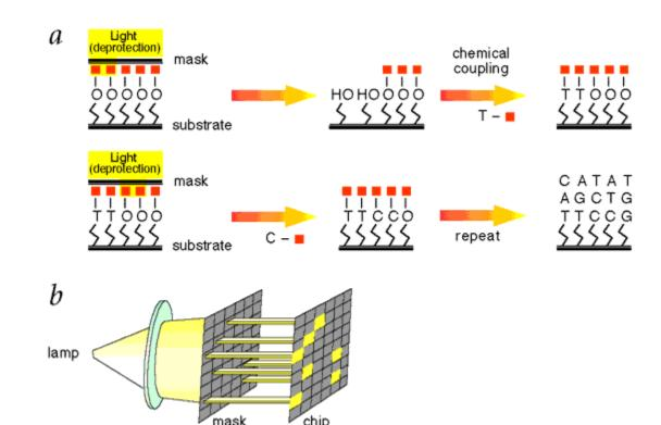
(a) Light directed oligonucleotide synthesis. A solid support is derivatized with a covalent linker molecule terminated with a photolabile protecting group. Light is directed through a mask to deprotect and activate selected sites, and protected nucleotides couple to the activated sites. The process is repeated, activating different sets of sites and coupling different bases allowing arbitrary DNA probes to be constructed at each site. (b) Schematic representation of the lamp, mask and array.
