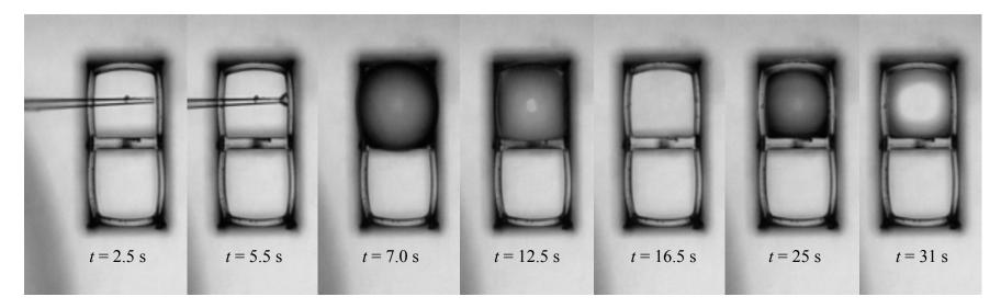
Filling the chambers of the structure shown in Fig. 5 with water using a 10 $\mu$ m diameter pipette. The top surface of the water is convex at t = 7.0s, flat at t = 16.5s, and concave at t = 25s.
