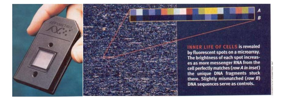
DNA chip can sense the state of up to 400,000 genes in a tissue sample. The number of probes on a single glass wafer may soon exceed 60 million, in which case the entire human genome will fit on 200-300 wafers.
