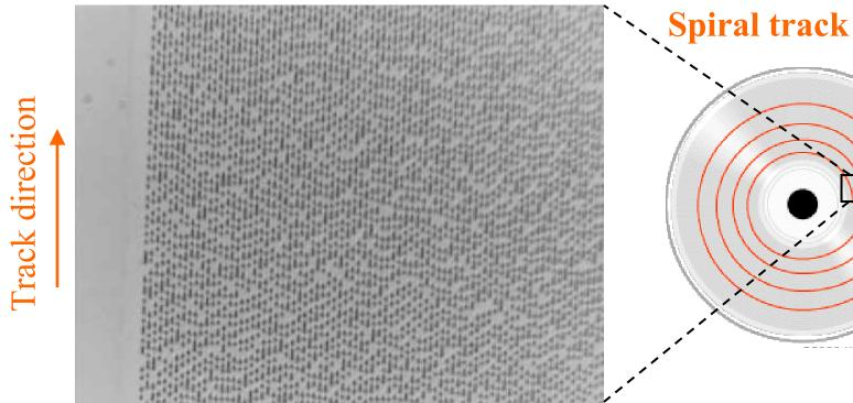
Low-magnification (×32) image of a CD showing an edge of the data zone.
