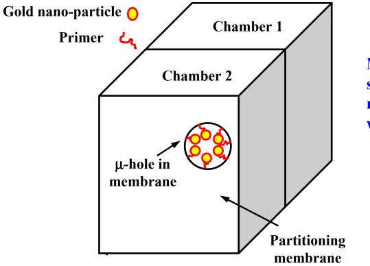
Method of forming a solidstate nano-pore in the micron-sized perforation within a partitioning wall.
