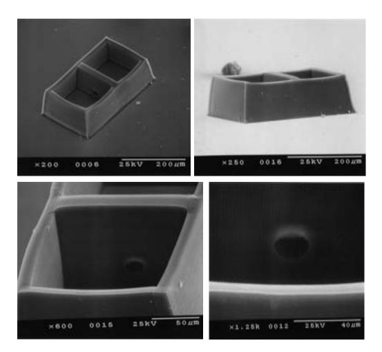
Two views of the microchamber fabricated by twophoton lithography. Each chamber is approximately 150µm on each side, and 150µm deep.
