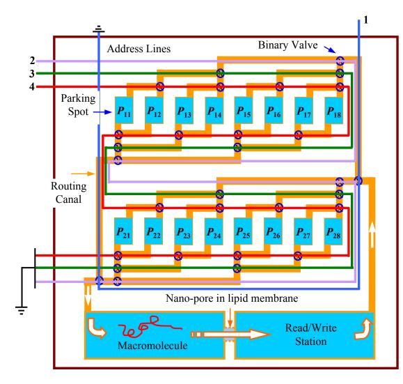
**Diagram showing the** patterned surface of the proposed data storage chip. **Once a parking spot is** selected, its macromolecular content will be transferred to the **Read/Write Station under** the influence of an applied electric voltage (i.e., electro-phoretic transfer). Following the completion of the read/write operation, the macromolecule should be returned to its designated parking spot.
