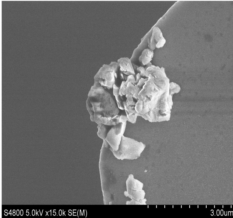
FESEM image of a  $\text{Si}_3\text{N}_4$  particle mounted on an AFM cantilever
