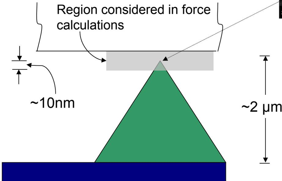
Geometry considered in modeling the force between nanoscale cantilevers and substrates
