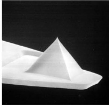
Sharpened silicon nitride probe
