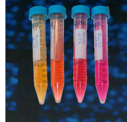
Phenol red is a common additive to cell culture media and is used to qualitatively determine pH changes based on color change on the cell culture media.
