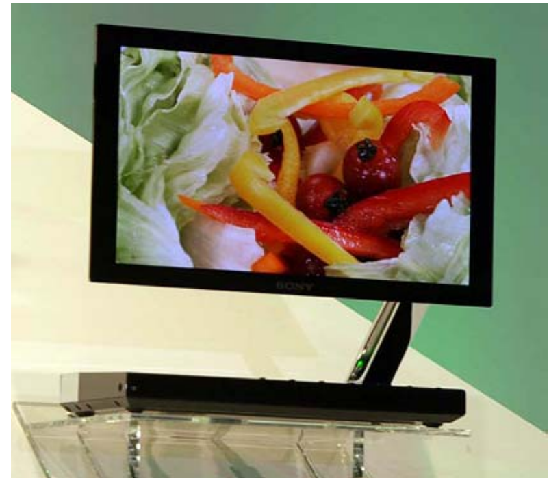
First OLED TV: Sony XEL-1 (Est. 40% less power than LCD)
