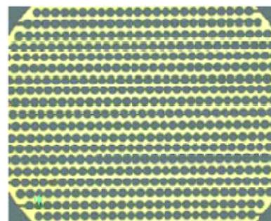
Circle-on-line microelectrode array
