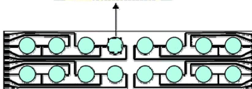
Microelectrode arrays on a glass slide
